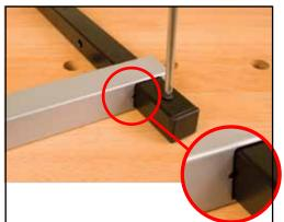
At the bottom one of the uprights (part #2) there is a screw hole 1/2" from the tip. Tighten one of the small sheet metal screws (part # 3) into the hole. Slide one of the shelf brackets (part #1) with the notched side (circled) of the bracket facing down.
