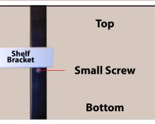
When Mounting to the wall the shelf bracket must be positioned as shown above, so that the small sheet metal screw is on the bottom of the shelf bracket.
